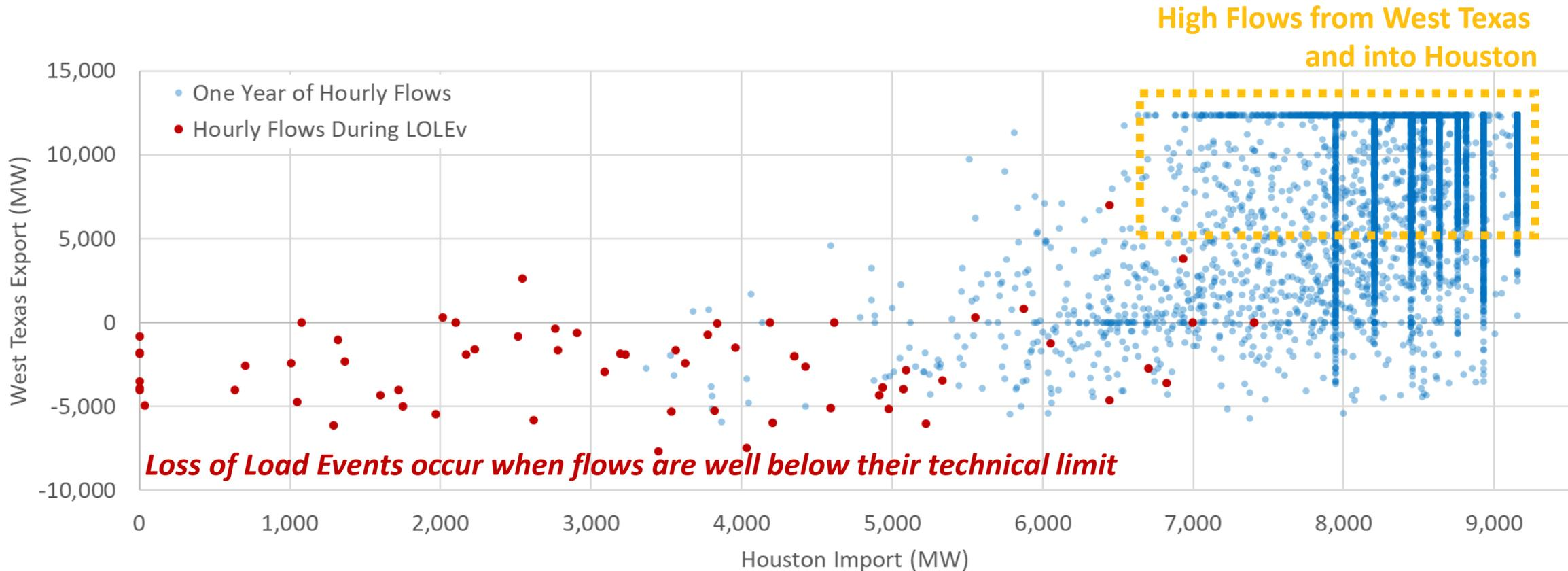
**Loss of load events occur when wind and solar output is low, and transmission interface has low (reverse) loading**
